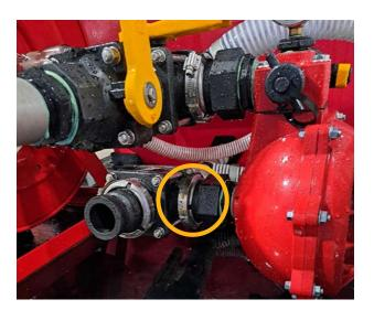
**Step 2:** Remove pump drain plug. **Step 3:** Tilt skid forward to drain tank.
