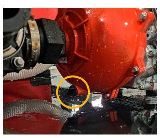
**Step 4:** Remove nozzle from hose on reel and blow air through the hose. Water will run out of pump drain hole. Blow air through hose reel until water no longer drains out of pump drain hole. Must tap Cap200 cap to fit your male air fitting tip.
